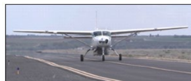
Boeing Cessna Caravan Autonomy Demonstrator Testbed carrying Safety Pilot, Flight Test Director, Caravan Rack Operator, for Remain Well Clear (RWC) Flight Test
